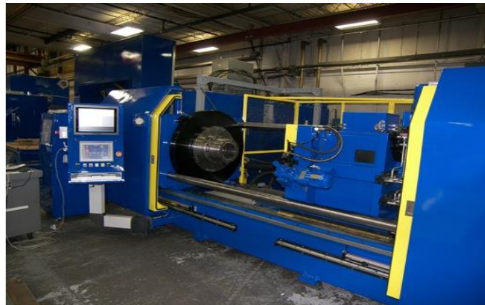
Inertia friction welding machine, MTC
